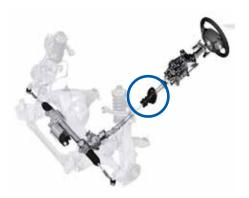
Steering column boot: covers the steering column in order to prevent dust and dirt from the engine room getting into the passenger compartment.
